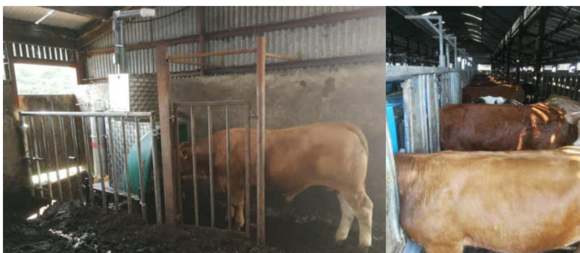
GreenFeed System estimating individual animal methane emissions
